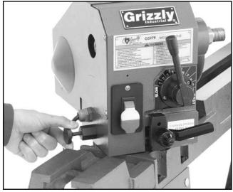
Figure 12. Adjusting headstock.
